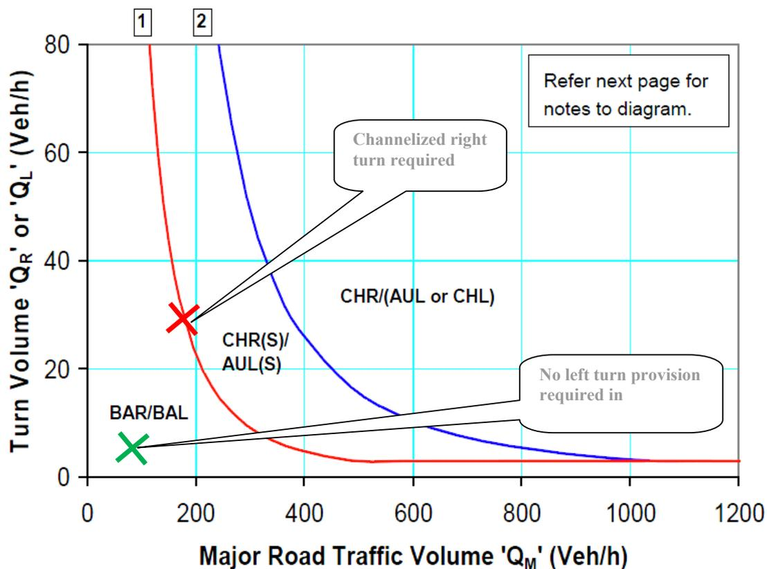
**Figure 4.1: Warrants for Turn Treatments on High Speed Roads - Construction**
